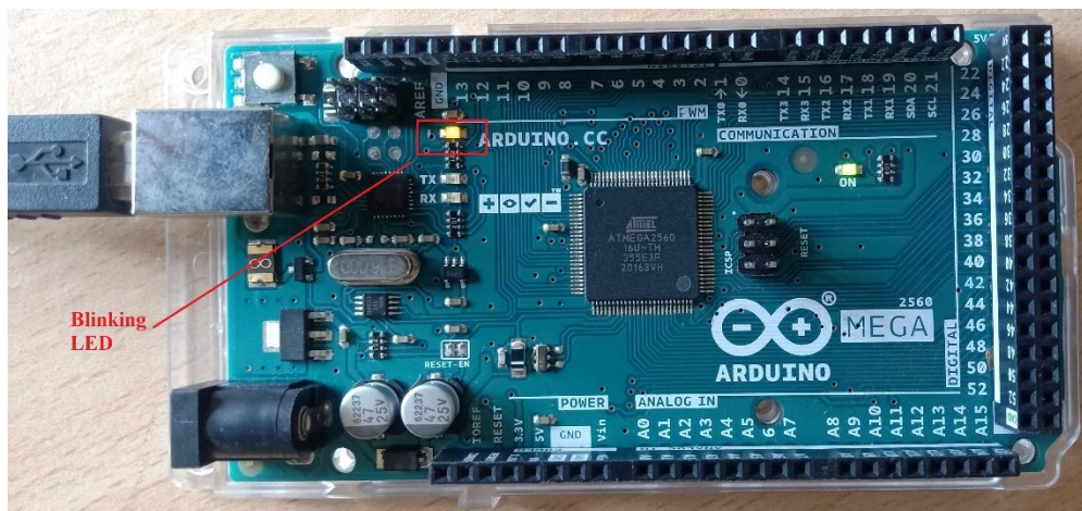
Fig. 9. Demonstration of blinking LED.
