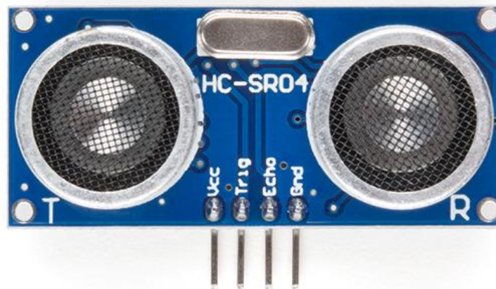
Fig. 13. Ultrasonic sensor with pins layout.
